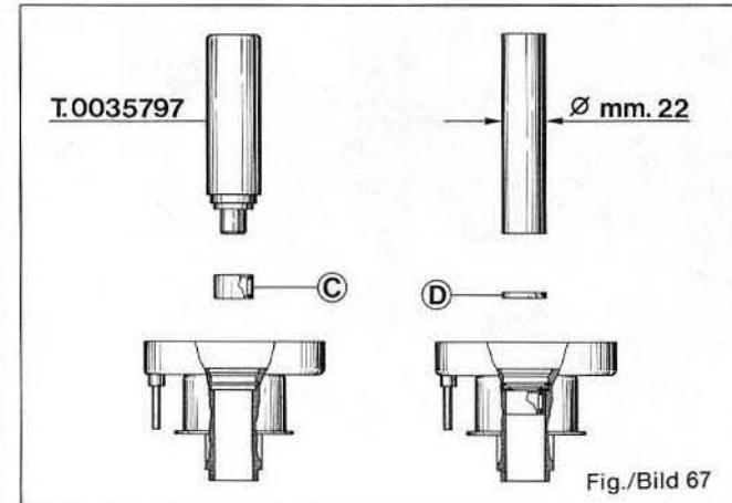
washers and 1 shoulder washer). The shoulder washer having a Ø 12 hole, should be fitted between both shim washers; then fit the circlips by using pliers T. 0017104 and with a Ø 26 mm. punch as shown position oil seal "B".
