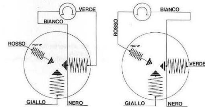
Connect the tester between the red cable and the white one in fig. 18; it should be measured continuity and ohmic value ( $56 \pm 5$  ohms). If after having checked the charge coil and the pick-up some anomalies come out, **replace the backplate or the damaged parts.**
