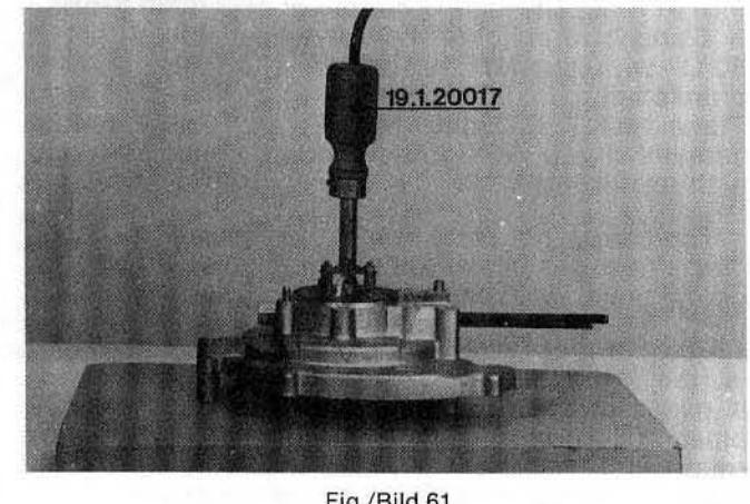
**Description of timing operations:** since coils are directly fitted on crankcase, timing check is limited to the verification that contact breaker points opening with the correct spark advance.
