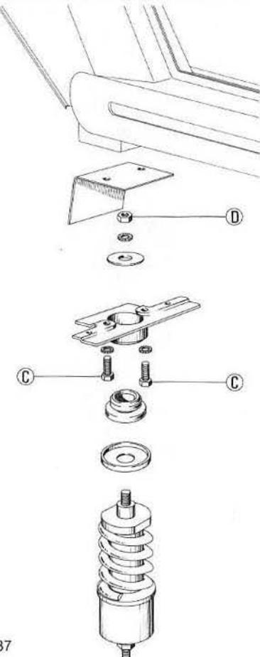
**Fig. 38 - Upper cone and front fork (Ciao - SI):** release the front brake cable, unloose both bolts securing headlamp to allow the loosening, by means of the 11 mm. wrench, handlebars securing tierod;
