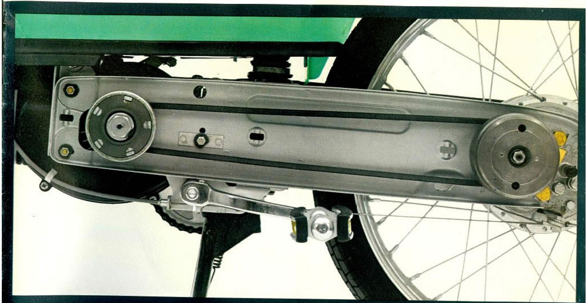
Full automatic transmission — Engine: single cylinder, two stroke, rotary distribution — To disengage the engine simply press this button and pedal away.
